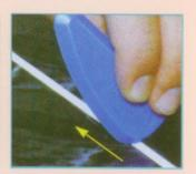
Choose the correct curve for grouting. Use the smaller or larger arc as desired. The sealent will be higher or lower in the groove depending on your choice.
